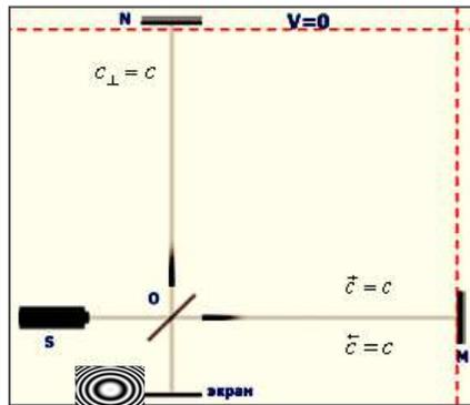
Fig 1 Rays come to the screen at the same time. In the center of the screen will be a bright spot.
