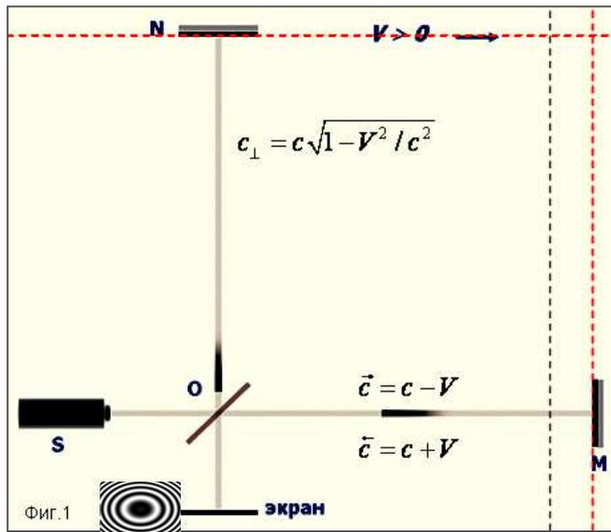
Rays come to the screen at different time. There is a phase shift. In the center of the screen a dark spot
